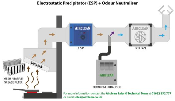
The Injection point of the odour neutraliser must be on the negative pressure side of the fan
